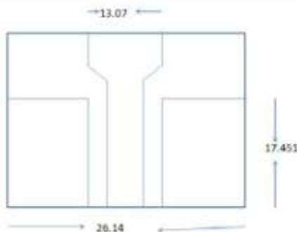
Figure.4 Geometry of proposed antenna
